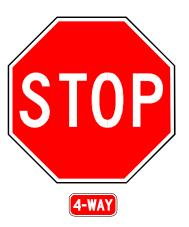
The installation of multi-way stop control must first meet the warrants as set forth in the MUTCD. Any of the following conditions may warrant an all-way STOP sign installation:
