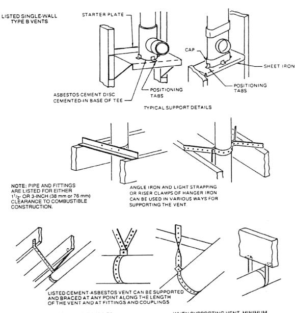
WHEN BASE OF VENT EXTENDS TO GROUND, IT SHALL BE SUPPORTED ON 2" (51 mm) OF SOLID MASONRY OR CONCRETE.
