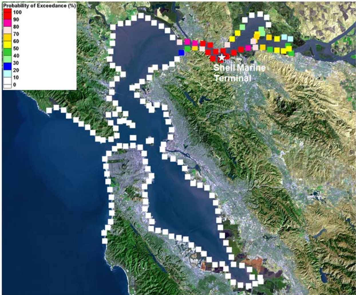
Figure A3. Scenario 3, Maximum Most Probable MT Spill, 168 Barrels, Shell Martinez Terminal, Summer
