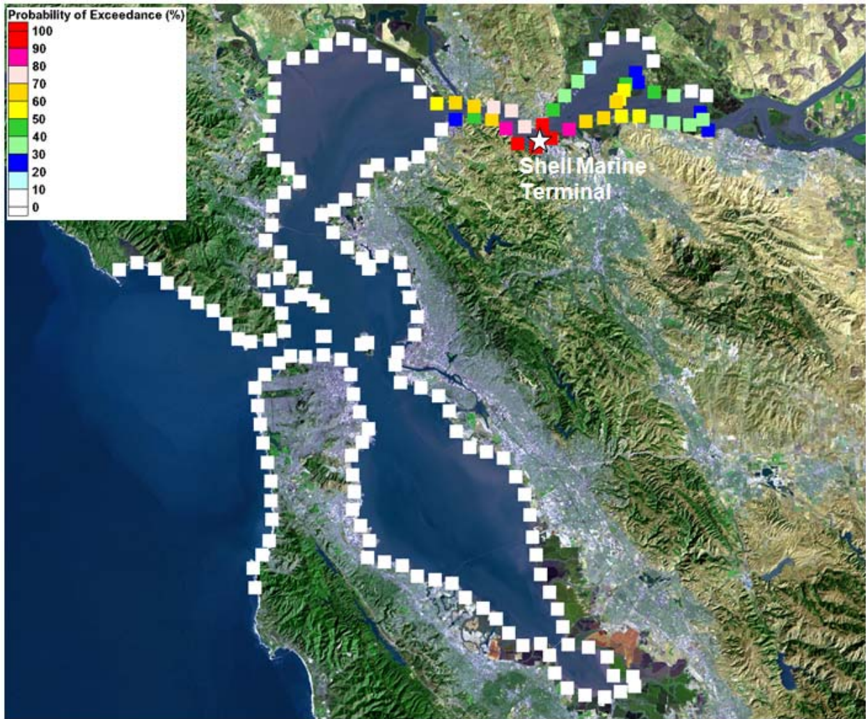
Figure A5. Scenario 5, Average Most Probable MT Spill, 50 Barrels, Shell Martinez Terminal, Summer
