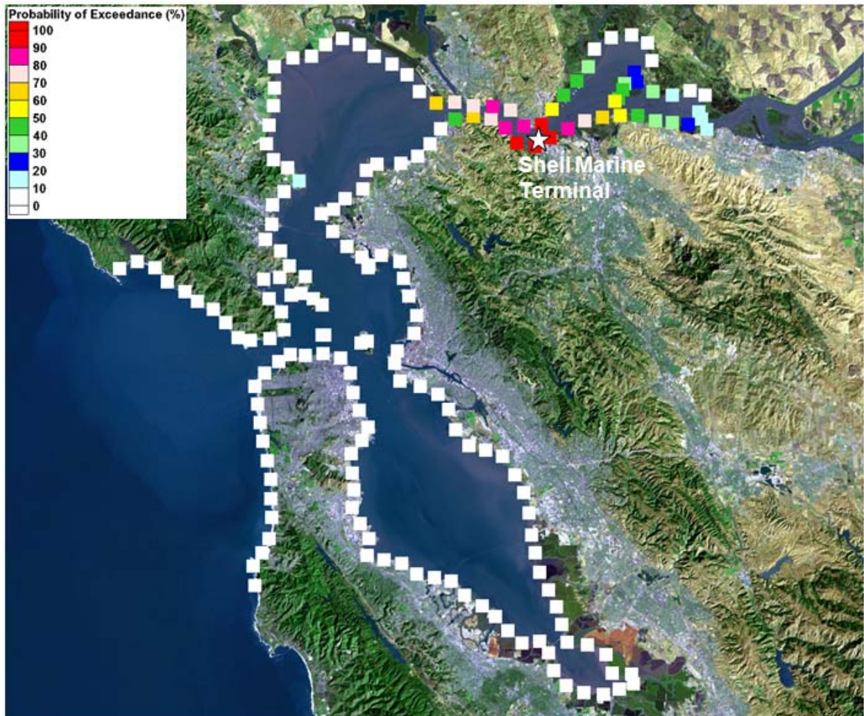
Figure A6. Scenario 6, Average Most Probable MT Spill, 50 Barrels, Shell Martinez Terminal, Winter
